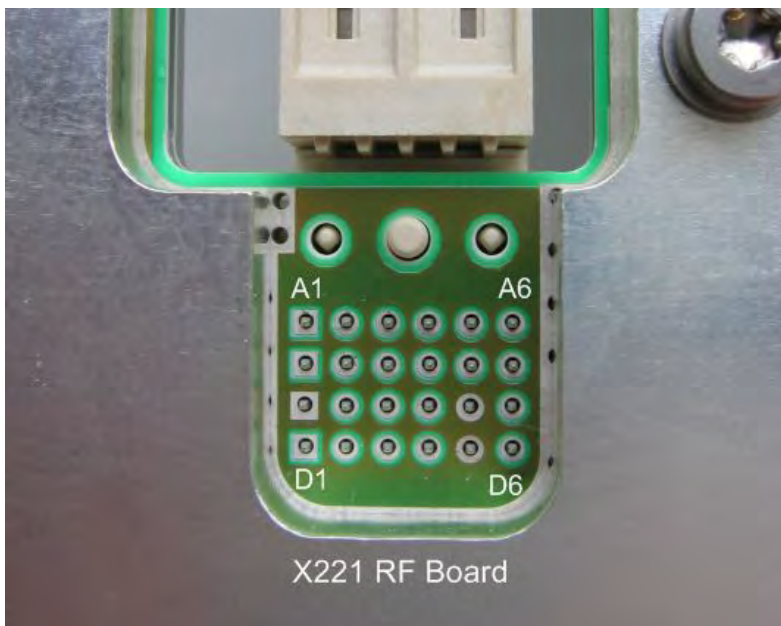
Fig. 3-10 Pin location X221 on RF Board
